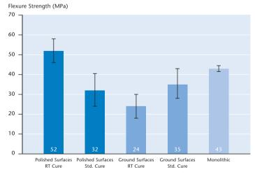
Measured on core drilled, fine ground specimens
